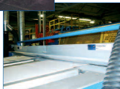
On a corrugator dry end, slit web cleaning before upper sheeting knife
