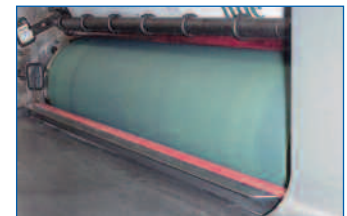
Blanket cylinder after 500 sheets with cleaner ON
