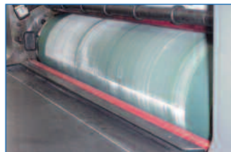
Blanket cylinder after 500 sheets with cleaner OFF
